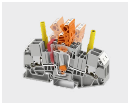
"Make before break" automatic leading current transformer short circuit for the test-disconnect terminal blocks
